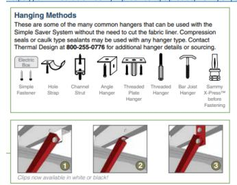
What is intended is for hangers to not protrude down from space and require large cuts in the fabric. We have had some contractors want to install their full hanger then have to overcut a large slit in the material and this will not be allowed. The preference is for the hanger to be either post installed through, or the hanger only hang down a short distance then coupled to extend down lower afterwards.
